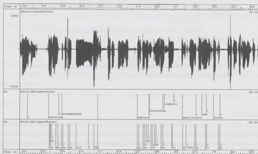
Figure 1 – An annotation example. At the top, the speech waveform; next, the orthographic annotation (words); at bottom, the phones where problem were detected.
